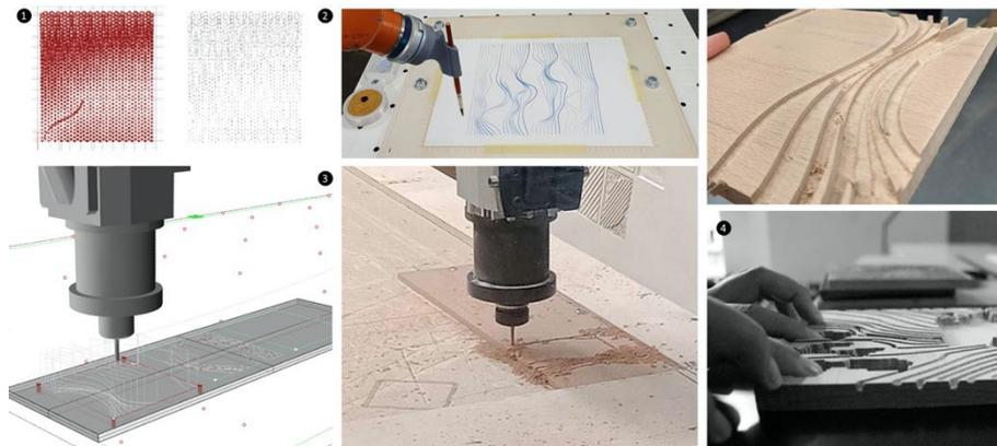
*Figure 4. Script with pixilation for image conversion (1), trial of robotic milling path based on line codes through drawing (2) and transfer to milling (3), with manual testing of tactile proficiency (4).*
