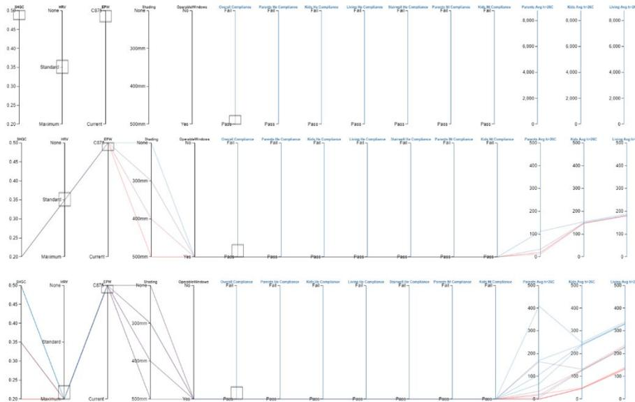
Figure 5. Top: For the baseline design parameters, the modelling could not produce a design that passes TM59. Middle: TM59 compliance could be achieved by decreasing the glazing SHGC Bottom: TM59 compliance could also be achieved by increasing the air change rate of the HRV
