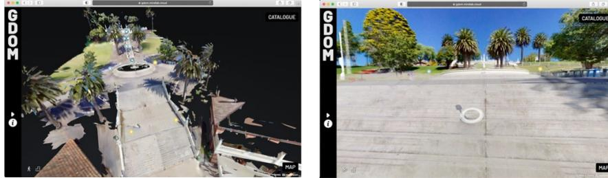
Figure 1: 3D mesh of GDOM Eastern Beach (left) and navigation of the corresponding 360° images using the crawling cursor (right)
