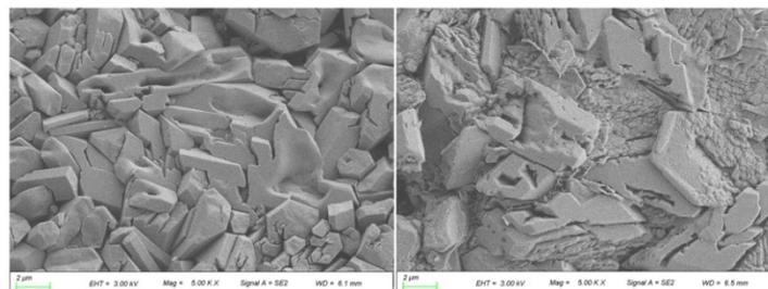
Figure 1. Left: Micro-structure of gypsum crystal without active excitation component (Group A)
