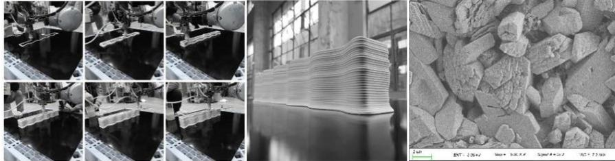
Figure 9. Print process and micro-structure of gypsum treated with modified components
