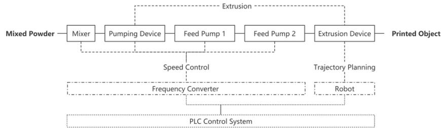
Figure 5. Robot-based gypsum 3D printing workflow diagram
