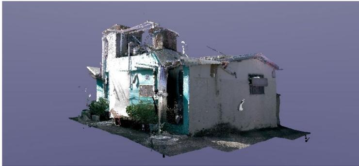
*Figure 8. Height extract form 3D point cloud registration*
