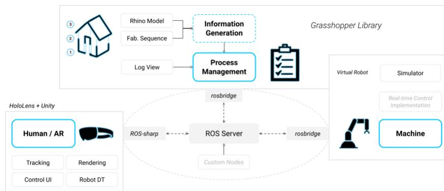
Figure 1. Augmented Reality Human Robot Collaboration System
