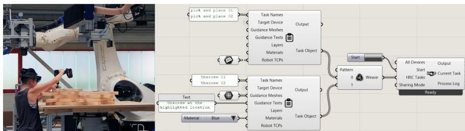
Figure 7: HRC Task Controller Workflow (Sequential Task Sharing)
