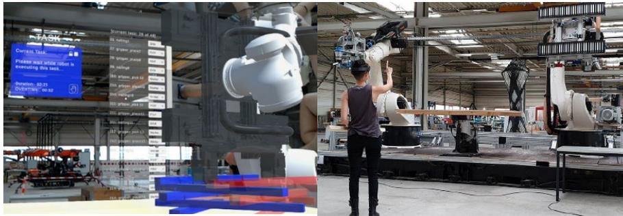
*Figure 8: AR interface showing the task information panel, task list, robot digital twin, and work geometries overlaid on the physical workspace (Left) and Craftsperson wearing HoloLens (Right)*
