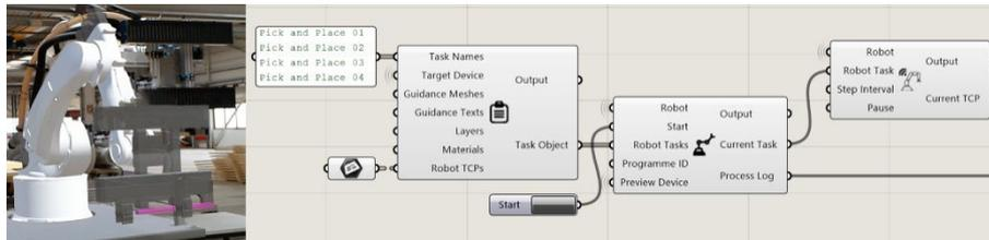
Figure 6. Robot Controller Workflow (Pick and Place Simulation)
