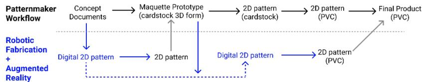
Figure 2. Diagram showing workflow between handcrafted techniques (black) and techniques using robotic fabrication and the AR interface (blue).
