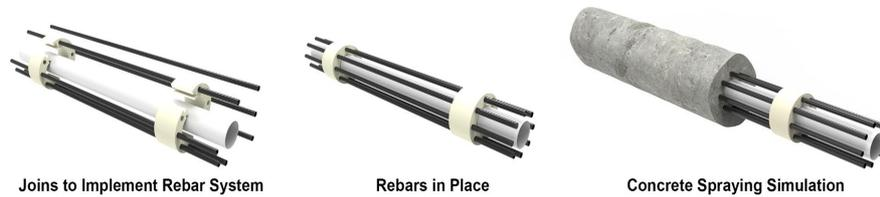
Figure 2. Construction System - PVC Pipes/Rebars/Joins
