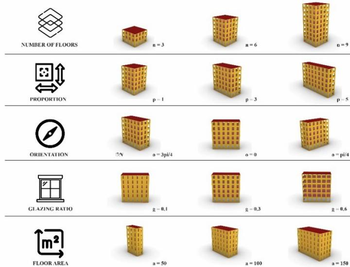
Figure 3. Parameters of a building archetype.
