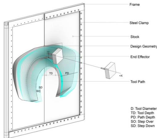
Figure 3. Robotic fabrication setup with a forming tool
