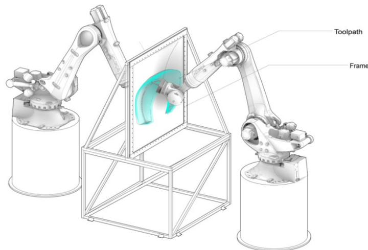
Figure 2. Robotic fabrication setup with two KUKA KR-210
