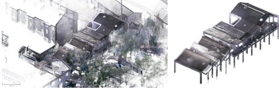
Figure 5. Registered point cloud of the building (left);
