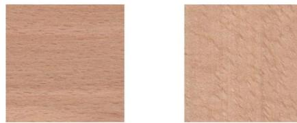
Figure 4. (Left) Spindles formed by the medullary rays run mostly parallel to the annual growth ring. (Right) Spindles formed by the medullary rays running mostly at an angle of 315° to the annual growth ring.
