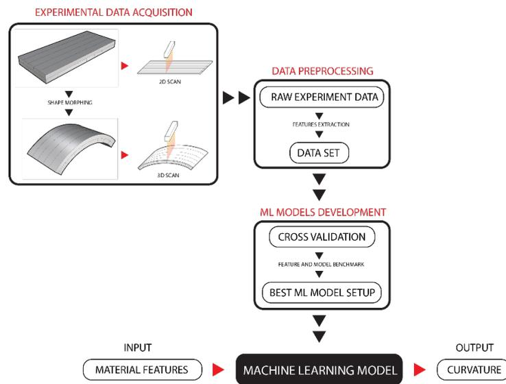
Figure 1. A flow chart of data-driven modelling for predicting self-shaping behaviour of wood bilayer. It includes bilayers sample production and data acquisition, data pre-processing, and ML models development.
