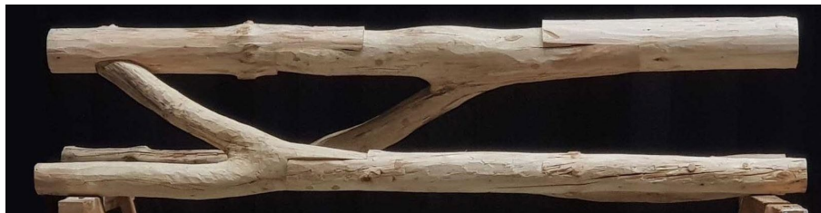
Figure 5: Assembly of the prototype using three tree forks and four straight segments.
